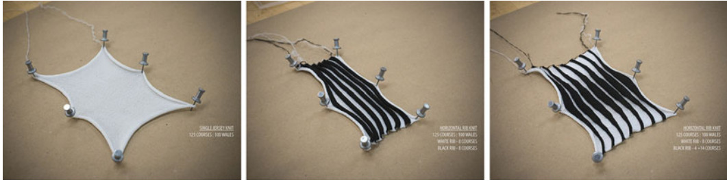
Fig. 9 Primary samples for studying basic single jersey behaviour to horizontal rib-knit and horizontal rib-knit with varied number of courses within each rib
