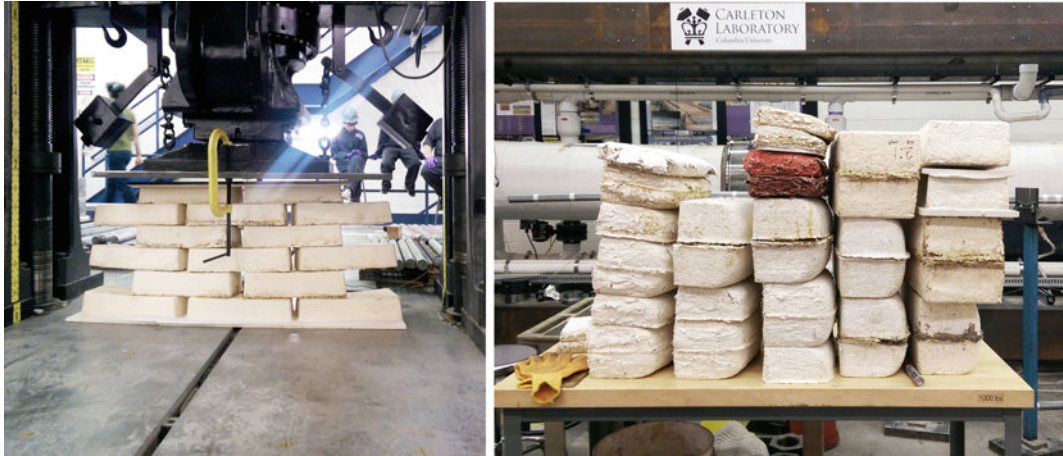
Fig. 3 Wall assembly being tested for performance under compression ( left ). Single bricks and composites before and after testing ( right )
