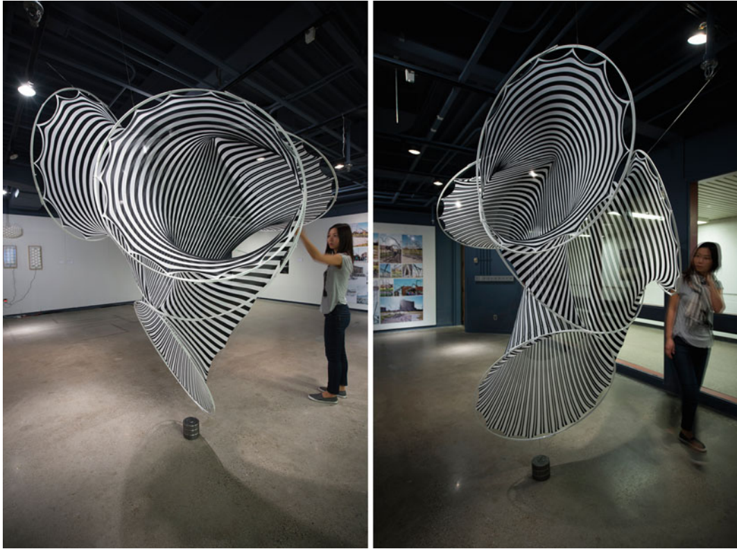
Fig. 1 Möbius Rib-knit prototype developed as a textile hybrid structural system, integrating glass-fibre reinforced rods and machine knitted textile; (Ahlquist 2014)
