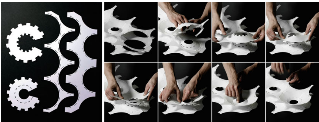
Fig. 10 The entire structure consists of four basic shapes that are clamped together by a local snap-through instability mechanism
