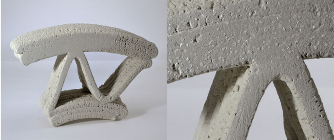
Fig. 6 Multi-material object printed with our system
