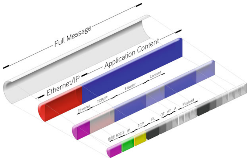
Fig. 2 Packet structure of a typical nested message generated by the library and shared over an Ethernet/IP network
