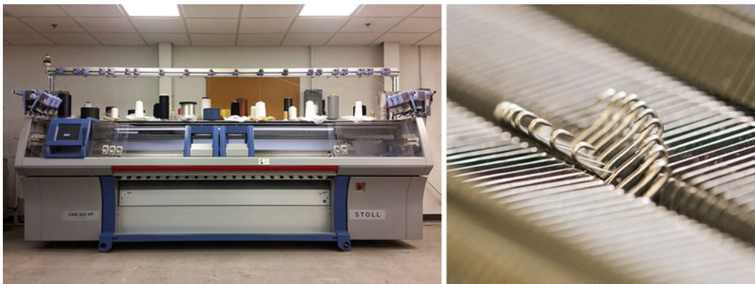
Fig. 3 Stoll v-bed knitting machine, 14 gauge with 82 needle bed, part of the FabLab facilities at the University of Michigan, Taubman College of Architecture and Urban Planning; (Ahlquist 2014)
