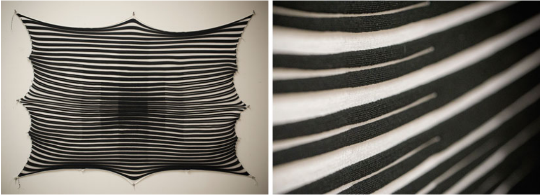
Fig. 13 Full scale knitted textile with bifurcating rib-knit structure for shaping; (Ahlquist 2014)
