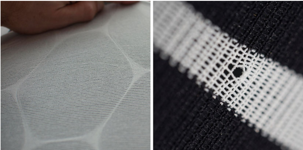
Fig. 14 Comparative resolution of designing textile behaviour, at the scale of the hexagon in the Semi-toroidal prototype versus the scale of the individual
