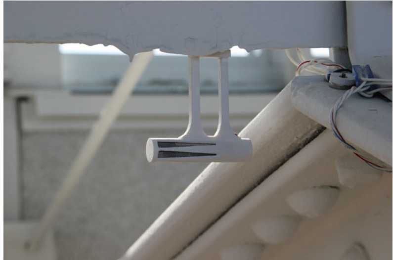
Fig. 7 Relative humidity sensor installed with integral magnets
