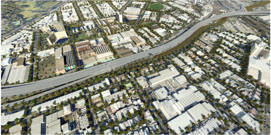
Fig. 4 Aerial perspective rendered view of Arden-Macaulay showing AURIN datasets, 3D photogrammetry building geometry with procedurally generated high-polygon mesh proxy object trees. Image courtesy of White and Langenheim (2014)
