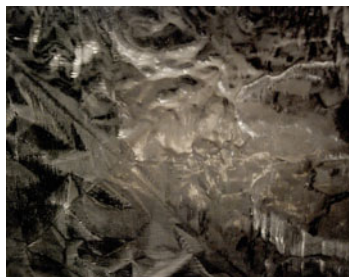
Fig. 19 Looping texture produces more dispersed light and opaqueness
