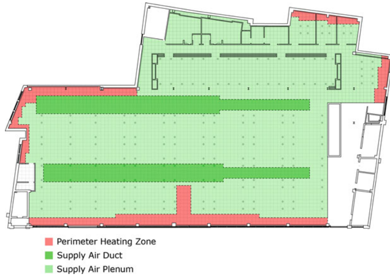
Fig. 11 Plan of raised floor system, indicating perimeter heating zones, supply air ducts, and supply air plenum
