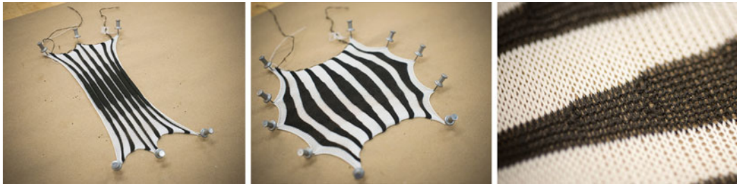
Fig. 10 Key parameters in designing textile behavior: directionality of stress along the length of the ribs, and varying width within each rib to shape the overall textile; (Ahlquist 2014)
