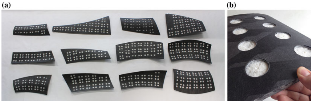
Fig. 7 Sandwich formwork composite with blind hole. a Different components. b Close up
