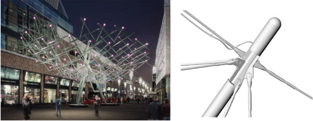
Fig. 4 Rendering of one of the original tensegrity structures in The Hague (left), Architect ELV Architecten © Studio i2, and model of the conventional structural node and light fixture, linking six cables and strut (right)
