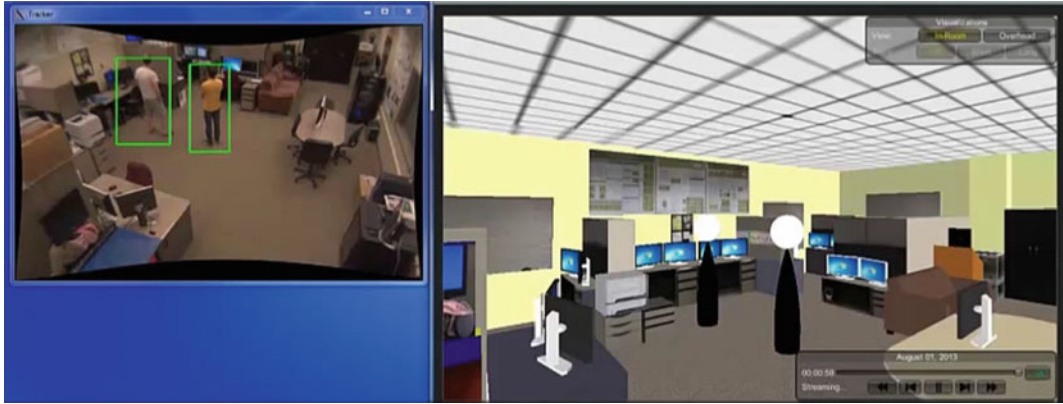
Fig. 1 Camera view of setting and avatar representation. Multiple camera views are resolved into a single model for analysis. Note the anonymous nature of the avatar view
