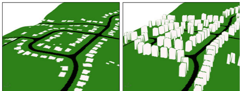
Fig. 3 Single 3d site information mesh before and after integrating elevation vector data
