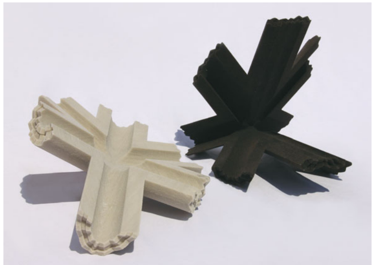
Fig. 5 EZCT Architecture & Design Research, 2013. Studies in recursive lattices, detail of the structure with thinnest section of 3 cm diameter
