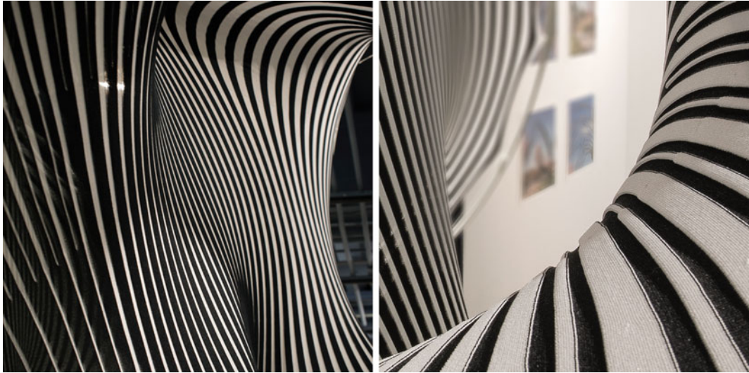
Fig. 15 Controlling the relationship of internal knit behaviour and global stress distribution, moments within the textile surface are allowed to maintain their dimensional rib-knit geometry; (Ahlquist 2014)
