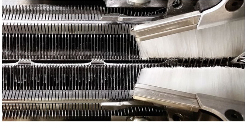
Fig. 6 Detail of vertical rib-knit structure on knitting machine; (Ahlquist 2014)
