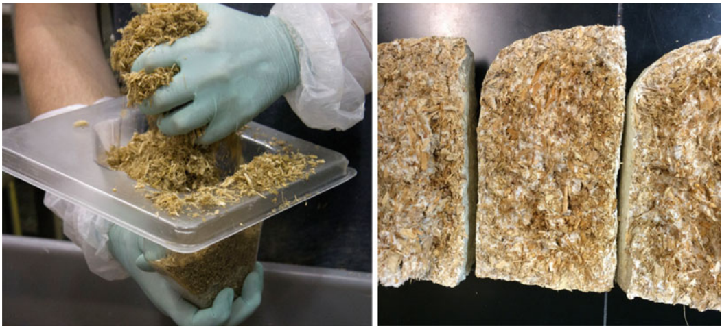
Fig. 7 Internal composition of bricks, consisting of a loose fill of crushed corn stalks and hemp
