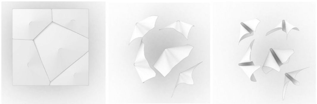
Fig. 20 Simulation of surface, randomly subdivided into sheet elements from planar geometry through continuously variable adjusted states to fully closed 3D-state
