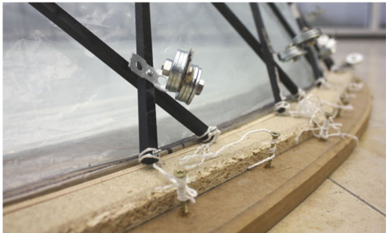
Fig. 6 Comprehensive edge beam detailing which includes clamping strips for membrane lip, support positions with channels to feed support cables and anchorage (screw) for the cable
