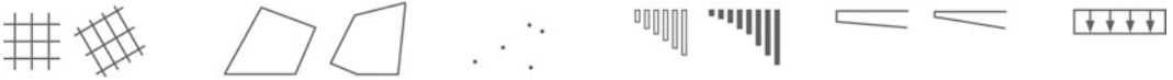
Fig. 10 Cross sectional variation—input: initial grid, outline, support location, cross section range and stiffness distribution, edge member cross section, loads
