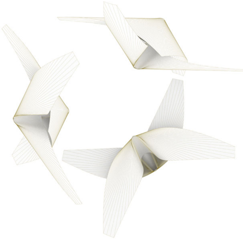
Fig. 1 Visualization of six simulated, additively arranged sheet elements in fully closed state
