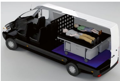
Fig. 12.5 Schematic of the mobile simulation unit shown in Fig. 12.4 is designed to accommodate stretchers, simulation equipment, clinical equipment, and the education team that will perform the training. (Photo courtesy of eSIM Provincial Simulation Program, Albert Health Services)
