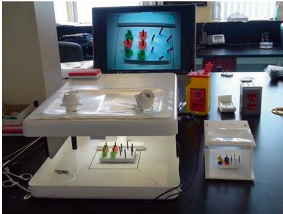
Fig. 22.4 A comparison of the adult FLS simulator to the PLS system. The pediatric simulator is smaller than the adult simulator by a factor of 20. PLS pediatric laparoscopic surgery, FLS fundamentals of laparoscopic surgery. (Image provided by: Dr. Georges Azzie MD, Assistant Professor, Sick Kids Hospital, University of Toronto, Toronto, Ontario, Canada. Reproduced with permission)
