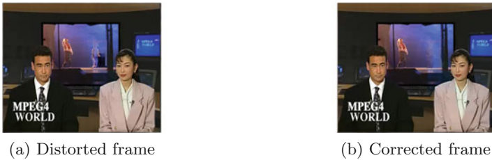
Fig. 3. An example of visual distortion due to DPM decoding error and its corrected version.
