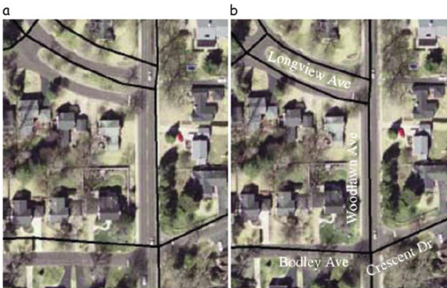
Fig. 9.34 Matching between road vector map and orthoimagery, from [123], Geoinformatica ©Springer 2006. (a) Map and image not aligned. (b) Map and image aligned
