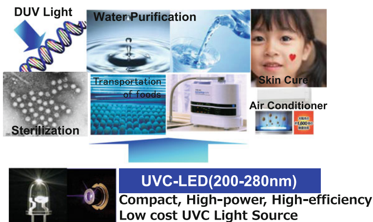
Fig. 4.1 Image of sterilization applications of deep-ultraviolet (DUV) LEDs
