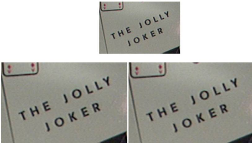
Fig. 3. When scaling ratio is 1.57, (a) original image (above), (b) the resized image by bi-cubic without any constraints about the coefficients of scaler (left), (c) the resized image by bi-cubic with N = 5 (right).
