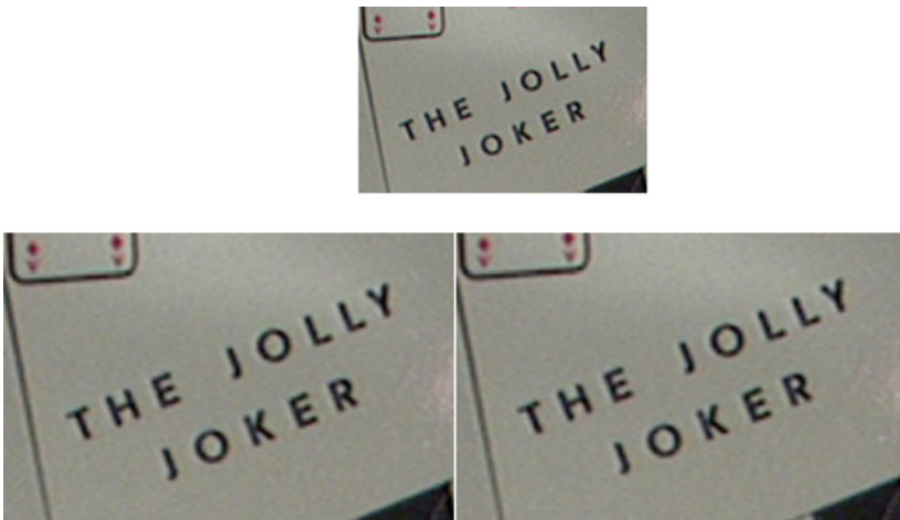
Fig. 5. When scaling ratio is 1.57, (a) original image (above), (b) the resized image by bi-cubic without any constraints about the phase (left), (c) the resized image by bi-cubic with M = 32 (right).
