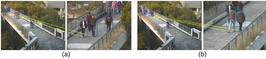
Fig. 1. Examples of tracking results in our dual-camera system. The left images in (a) and (b) are from the static camera, and the right images in (a) and (b) are from the active camera. Same persons moving in static and active cameras are linked with yellow solid lines (Colour figure online).
