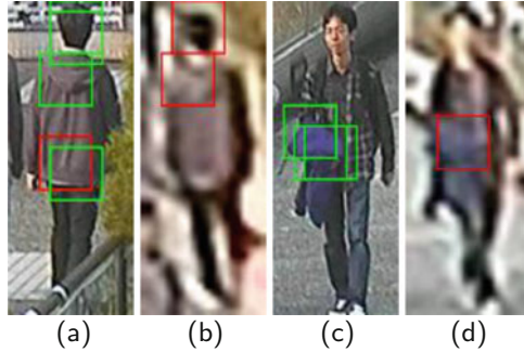
Fig. 3. Examples of the most discriminative features selected by static appearance models and active appearance models for two targets. (a) and (c) is the most discriminative features selected by active appearance models for target a and target b respectively. (b) and (d) are the corresponding discriminative features selected by static appearance models. The color and HOG descriptors are indicated by red and green bounding boxes, respectively.
