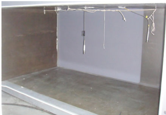
Fig. 7.8 Acoustic cavity with a steel plate partially treated by melamine foam; note the three receiver pressure microphones
