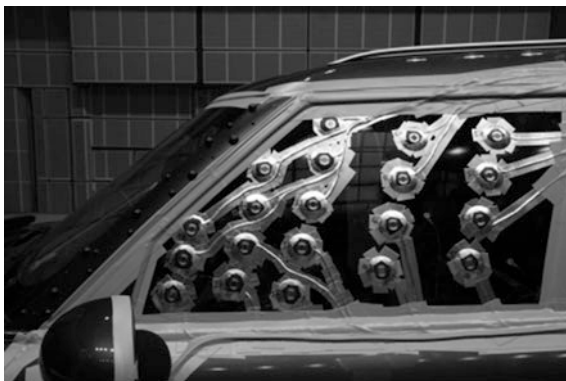
Fig. 1.3 20 surface microphones almost equally distributed on the side window
