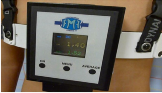
Fig. 17.9 Measurement of the Pressure Of Treatment (POT). Before and after adjustments to the FMF ® DCS. Note the three buttons for optimum performance and the digital multiparameter color display of the Pressure Measuring Device (PMD)
