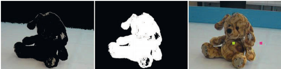
Fig. 6. Inner space and object detection, center of gravity (yellow), desired position (pink)
