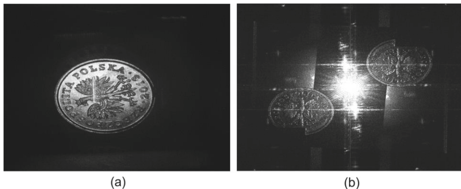
Fig. 4. The results obtained from the holocamera with SLM: intensity images of the coin reconstructed from: (a) Fresnel hologram, and (b) Fourier hologram.
