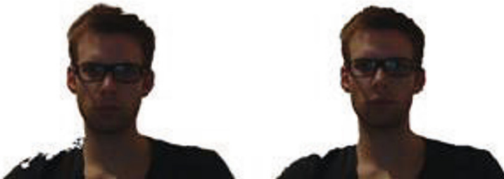
Fig. 3. Process result without (left) and with (right) GrabCut algorithm
