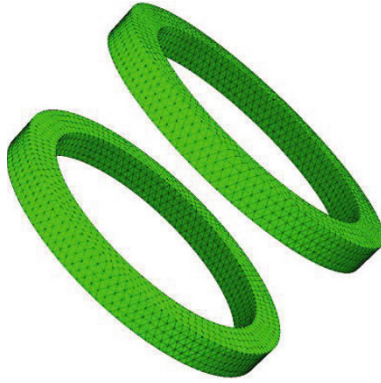
Fig. 1. Meshed model of Helmholtz coils utilized for simulations
