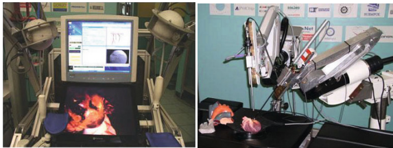
Fig.1. Teleoperator Robin Heart 1 and Robin Heart Vision during experiment electrocoagulation of wall of the heart. The effectors are similar to minimally invasive surgery instrumentation
