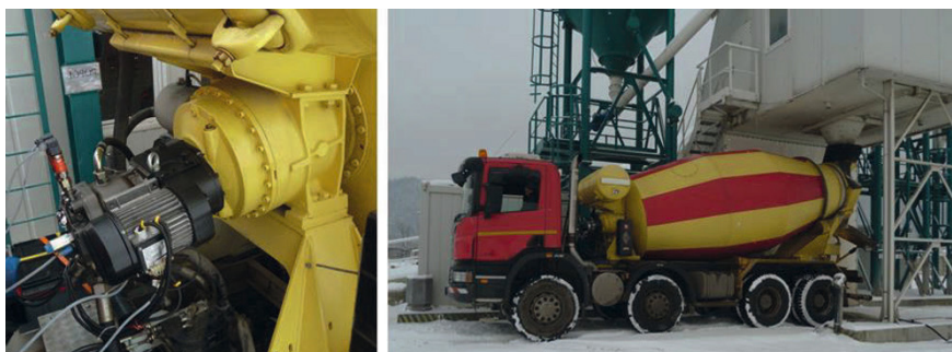
Fig. 2. Concrete Transit Mixer Application and prototype of hybrid drive unit
