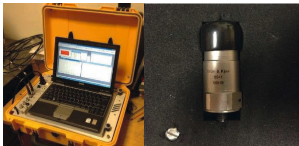
Fig. 3. „Brüel&Kjær“ machine diagnostics Toolbox – “Type 9727”; a) diagnostics toolbox, b) accelerometer “8341”
