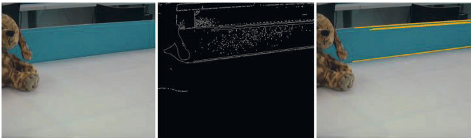
Fig. 4. Border detection using edge detection and Hough transformation
