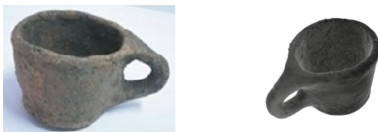
Fig. 2. A picture and NR-CT reconstruction of outer surface of the burial cup.
