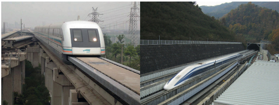
Fig. 1. Commercial Mag-Lev solutions: Transrapid (EMS suspension), Japan Railways Company (EDS suspension)
