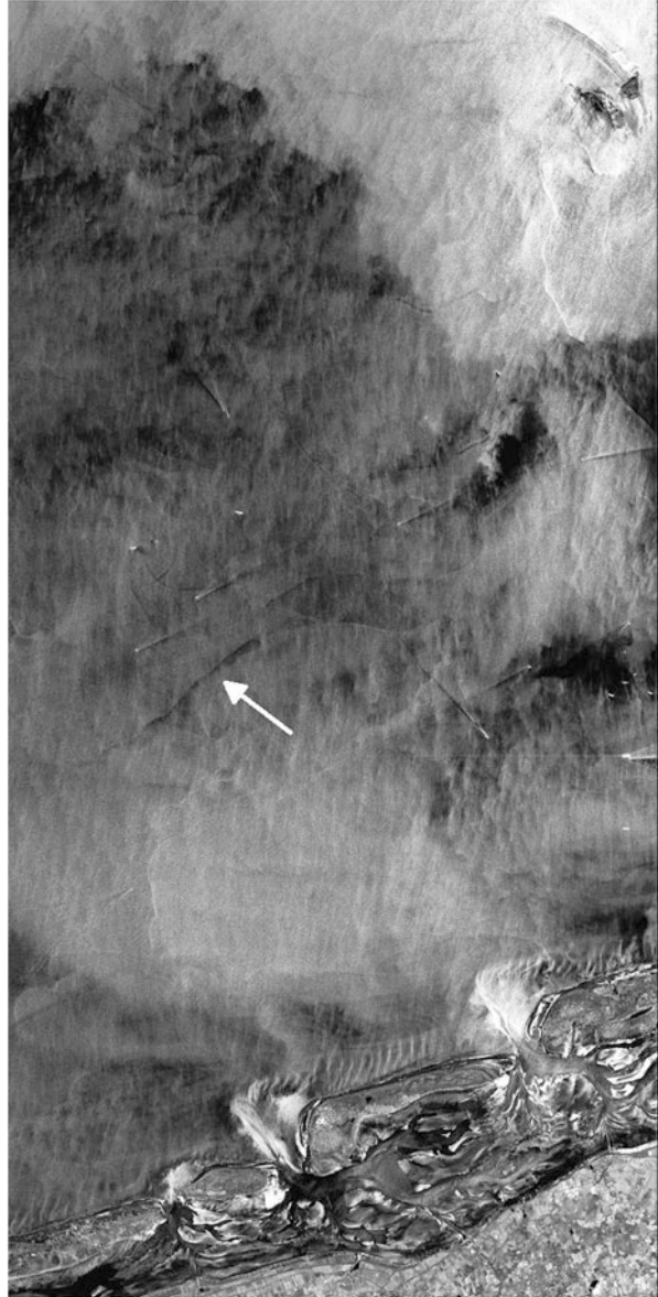
Fig. 6 TerraSAR-X image (StripMap mode, dimensions 35 \times 70 km) acquired on 9 February 2013 at 05:59 UTC and showing the German Bight, between the Helgoland island ( upper right ) and the German mainland coast ( bottom ). A number of ships, both travelling and anchoring, can be seen in the image centre. The arrow marks an elongated feature, probably caused by an oil spill © DLR
