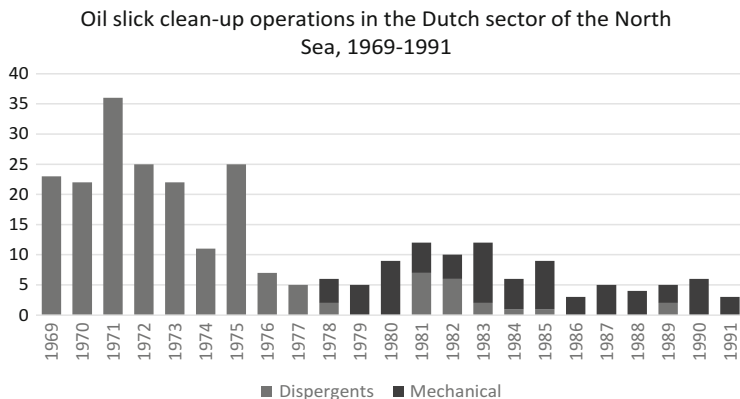
Fig. 4 Cleanup operations (n) in the Dutch sector of the North Sea, 1969–1991. Note: Initially, oil slicks were sprayed with dispersants only. New mechanical techniques to combat oil pollution were introduced in the late 1970s, and these techniques were preferred in later years. From monthly and annual reports produced by the Ministry of Transport and Public Works [37, 38]
