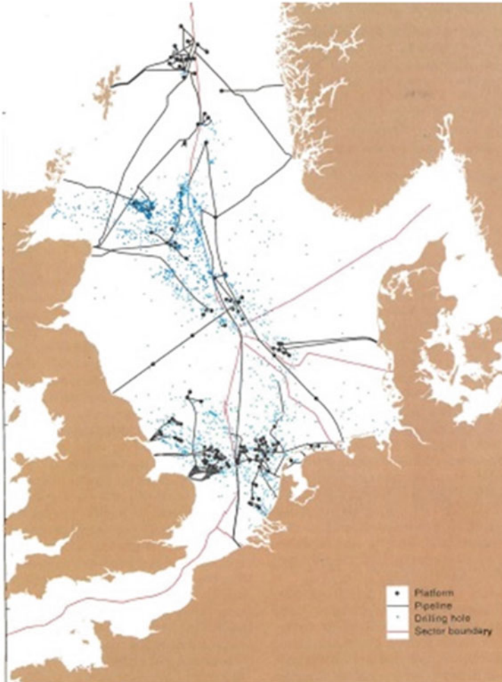
Fig. 2 Oil and gas production pipelines in the North Sea, 1991. Source: North Sea Quality Status Report 1993 [4, Figures 1–10, p 17]. Note: This figure shows oil and gas production platforms and pipelines in 1991, together with the position of oil wells and exploration drillings
