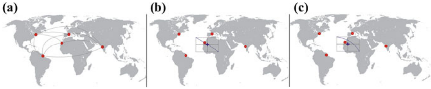
Fig. 5.2 Methods to measure dispersion of geolocated points ( red dots ) on a map. a Average of pairwise geodesic distances between points. b Diagonal of the bounding box defined by the standard deviations of latitude and longitude around the center of gravity ( blue cross ). c Same as ( b ) but considering the geodesic distance of the diagonal
