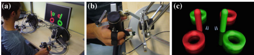
Fig. 3 Experimental setup. a General overview of the setup. b Detail of one hand wearing the cutaneous devices. c Virtual environment with surgical pliers
