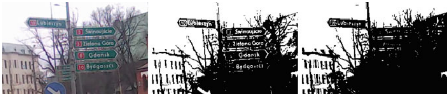
Fig. 1 An exemplary natural image with results of its Otsu binarization for CIE LAB and YUV luminance channels (from left to right respectively)
