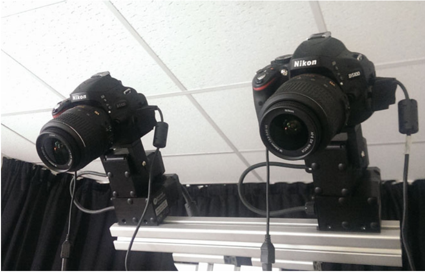
Fig. 1 The active stereo head used in the experiments
