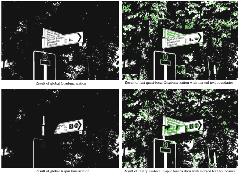
Fig. 3 Comparison of the results of global and fast quasi-local binarization for an exemplary image from the NEOCR dataset
