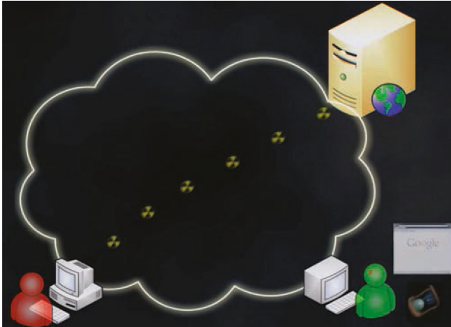
Fig. 1. DoS attack execution. The attacker is labelled red and a huge amount of special requests are sent to the server to make the service unavailable to other legitimate users (labelled green), adapted from Internet [15] (Color figure online)
