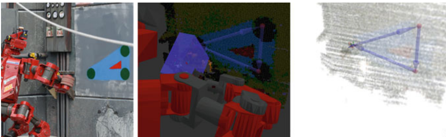
Fig. 3 CHIMP preparing to cut a triangular pattern from a wall in the DRC Trials, along with a Box fixture representing the volume of the drill in the hand, and a PlanarPath fixture showing the triangular shape to be cut
