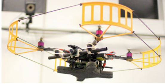
Fig. 1 Our quadrotor experimental platform equipped with a Intel NUC computer, a MEMS IMU, and a camera. This quadrotor can be launched without initialization at a preferred state. It can autonomously maneuver through different trajectories, and recover from possible failure conditions on-the-fly
