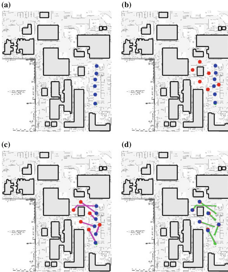
Fig. 8 A series of snapshots of the user interface while running an experiment with six robots. a Initial positions, b user species goal positions, c planner assigns the goals and generates trajectories, d actual trajectories followed by the robots
