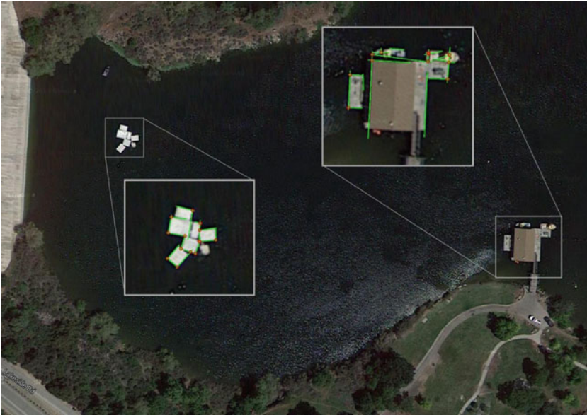
Fig. 4 Detected calibration sites in experimental area. Green lines indicate the detected lines and red circles indicate detected corners
