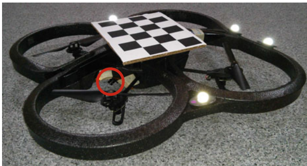
Fig. 4 The AR.Drones are equipped with a checkerboard and Vicon markers for relative sensing and ground truth poses, respectively. The forward-looking camera is tilted 45° downwards (highlighted by a red circle) to track the target and robots on lower levels of the sensing topology
