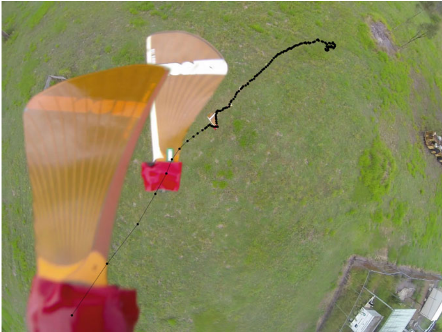
Fig. 5 Sensor descent trajectory montage. Tracked point is the centre of the sensor module in each frame, at 50 fps
