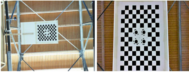
Fig. 5 Influence of camera mounting on marker detection tolerance. The pictures show the marker as seen from the camera for way-point 1 in environment ALU-FR. Left Reference robot P3-DX, the camera is mounted at a height of 0.45 m, see also Fig. 1 (left). Right Freiburg's omniRob, the camera is mounted 90° rotated with respect to the camera of the reference robot and at a height of 1.7 m, see also Fig. 1 (middle)
