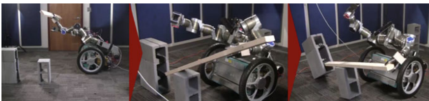
Fig. 9 Golem Krang places the lever in the planned pose and overturns the 50kg load
