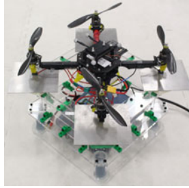
Fig. 5 Quadrotor resting on charging station
