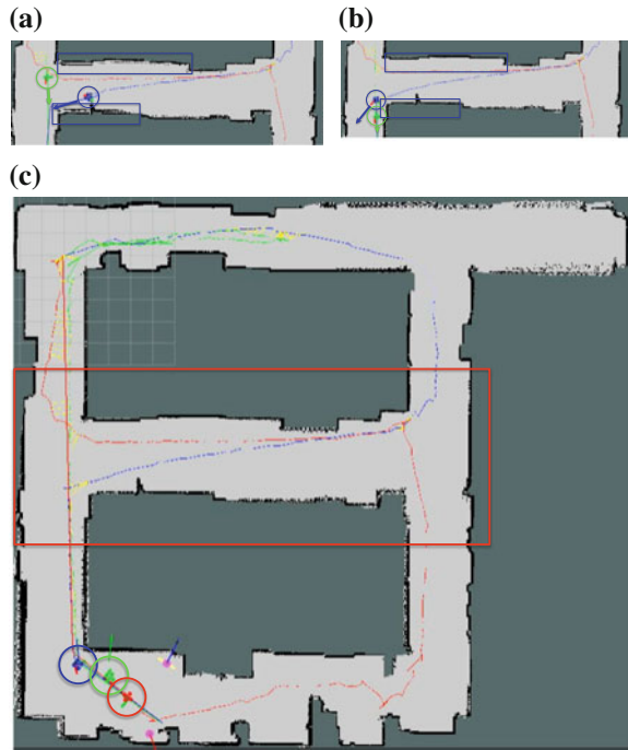
Fig. 8 Simulation of 3 robots exploring in an environment created from a prior 2-D map. Figure (a) and Fig. (b) shows the region inside red rectangular in Fig. (c). a Accumulated error results in spurious walls when multiple robots explore same area with large bearing differences, b odometry constraints between green and blue robots correct the map and spurious wall disappears, c after exploration done, we get a map which is almost the same as the prior map
