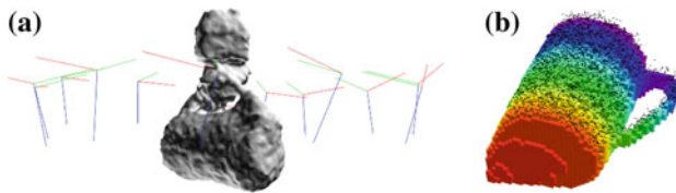
Fig. 7 a Thirteen registered views of a kettle held in the robot’s hand are used to carve a voxel grid, which is then meshed using Marching Cubes. The robot’s hand is reconstructed as well. b A coffee mug scanned by a simulated Kinect at a depth of 3 m in the intermediate stages of voxel carving. Voxels (colorful) are constructed from multiple noisy depth scans (black points)
