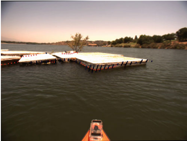
Fig. 7 Camera view with laser returns ( red dots ) and sonar returns ( dark blue dots or lines ) overlaid using transforms estimated by the calibration process. It is worth noting that since the floating platforms rise so low out of that water that the laser might not get a hit from the closest one. Also worth noting is that the overlaid sonar returns include the whole echo profile, not only the peak, which explains why they appear as lines
