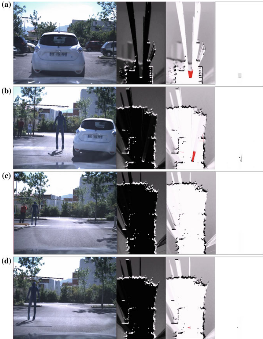
Fig. 8 Results of the system. Are presented each line a visual capture from the embedded camera, the estimated occupancy grid in front of the car ( white for occupied, grey for unknown, black for empty), the estimated motion field (if a case is seen as dynamic, a red motion vector showing the average velocity in the cell is drawn on the map) and finally the estimated risk map for 0.5 s. The first sequence a , b presents the appearance of an occluded pedestrian, the second c , d a moving pedestrian heading towards the road
