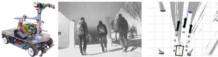
Fig. 2 Left platform used for data acquisition; middle sample image from a wide-angle camera; right sample of laser measurements showing three tracked subjects and their orientation as the dark vectors. The robot is represented as a black rectangle
