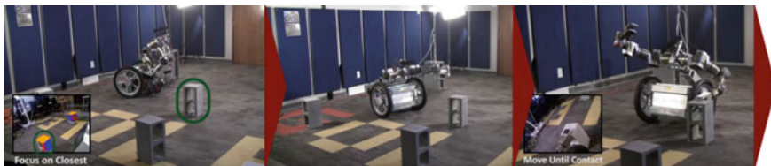
Fig. 6 Once Golem Krang detects the closest cinder block ( left ), it approaches ( middle ) and grasps the objects ( right ). Scene continues in Fig. 7
