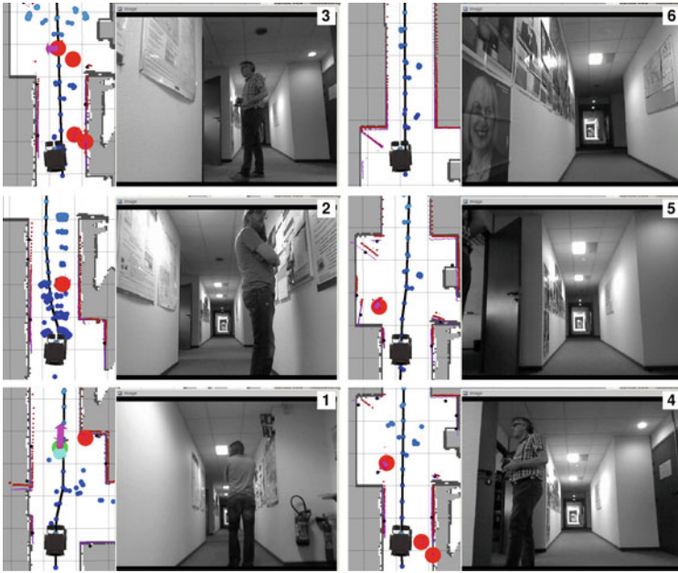
Fig. 14 Switching navigation method between leader following and independent navigation
