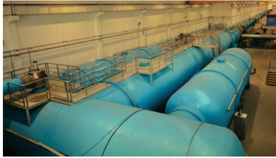
Fig. 10 Photo of long-test-duration hypervelocity detonation-driven shock tunnel
