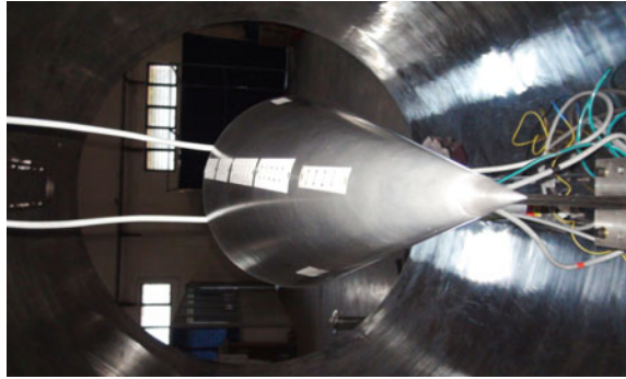
Fig. 36 A sharp cone model of 0.8 m length mounted in the test section of HST-4
