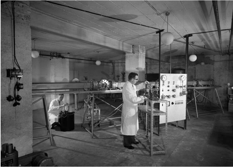
Fig. 18 Photograph of the shock tube of the Ernst Mach Institute having a test-section of 4 cm × 11 cm
