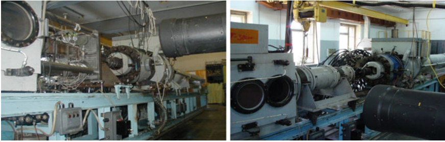
Fig. 4 General view of the IT-302 M hotshot wind tunnel; left, with a nozzle 300 mm in diameter and right, with an attached combustor
