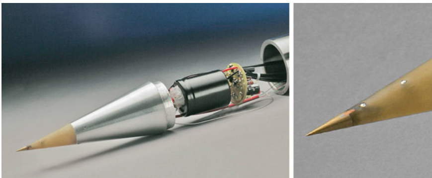
Fig. 33 Plasma-discharge actuator inside a 50-mm-diameter test model and a zoom on electrodes
