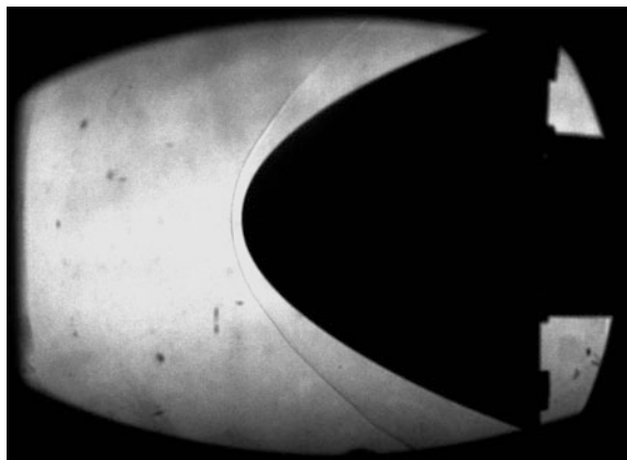
Fig. 12 Schlieren image of a hyperboloid installed in the test-section
