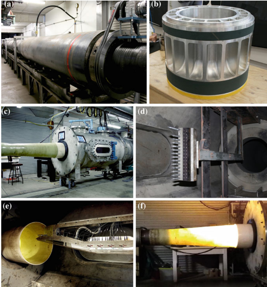
Fig. 21 Photographs of X3’s upgraded hardware. a Ø500 mm bore single stage driver compression tube (protective shielding removed to show capstan with belt drive). b Ø500 mm 100.8 kg lightweight piston. c Nozzle and test section with 50 mm thick perspex windows installed. d Pitot rake instrumented with 15° partial impact cone probes and a Pinckney static pressure probe [76, 85]. e Instrumented scramjet in test section (side covers removed). f Nozzle flash during facility operation due to flow luminosity [86]
