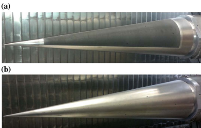
Fig. 28 Integrated cone model (from Wagner et al. [116]). a Porous insert. b Stainless steel reference surface
