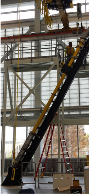
Inclined shock tube (under construction phase) showing platforms used for changing diaphragm
