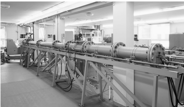
Fig. 20 Photograph of the 20 cm i.d. shock tube of the Ernst Mach Institute
