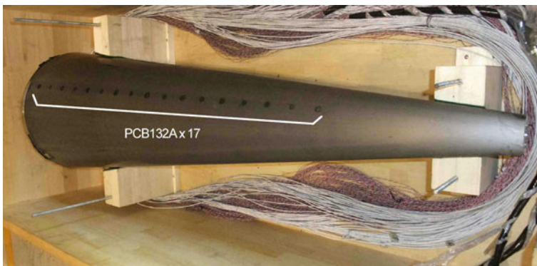
Fig. 41 7-degree half cone angle model equipped with 17 PCB pressure transducers for the second mode instability investigations
