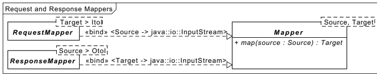
Fig. 3. The abstract Mapper class and its subclasses. Request mappers create inbound DTOs from input streams, whereas response mappers map outbound DTOs to technology-dependent client responses.
