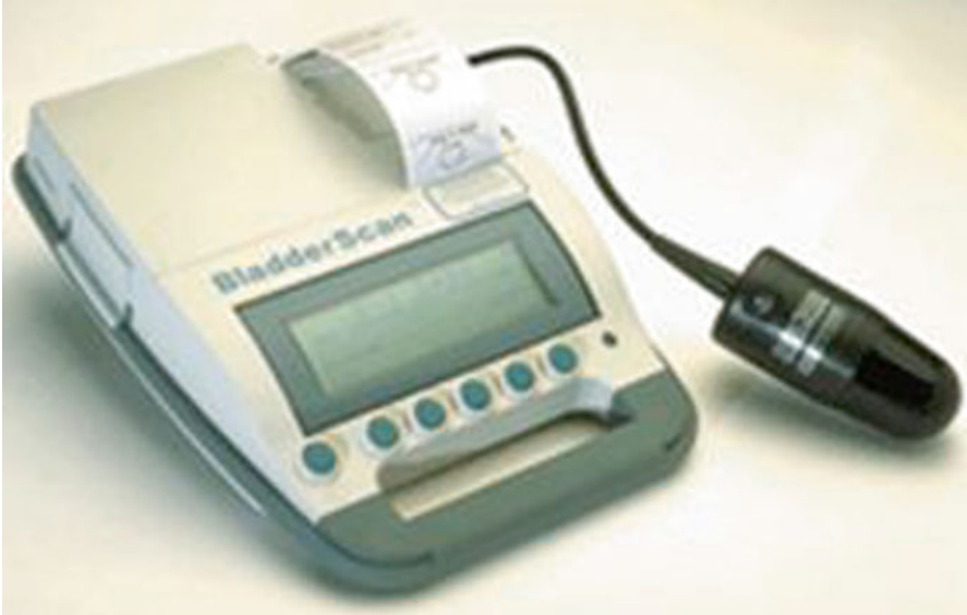
Fig. 3.2 Ultrasound post residual urine volume measurement machine
