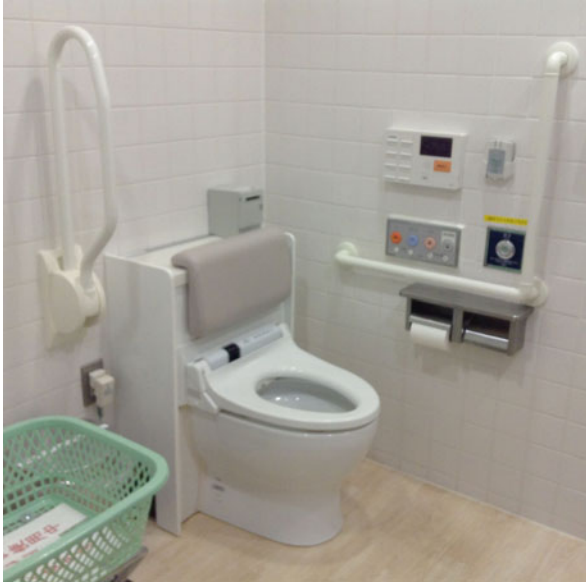
Fig. 3.9 Future flowmeter (Toto, Kokura, Japan). The next-generation uroflowmeter build into normal patient bathroom toilet in Doctor Tomohiro Ueda's specialty clinic in Kyoto, Japan
