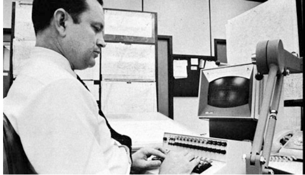
Fig. 2.1 C. L. (Chan) Chandler, Delta superintendent of weather analysis, keys in wind and weather data using IBM 2915 CRT linked to a 7074 computer. Image and caption source: Air Transport World magazine, March 1972
