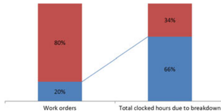
Fig. 3 Pareto analysis of clocked working hours of work orders related to breakdowns. As visualized, 20 % of the work orders with the most clocked working hours account for 66 % of the total clocked working hours related to breakdowns
