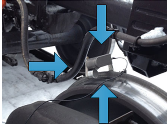
Fig. 3 Manual measurements performed with the hand-held MiniProf measurement equipment on an iron ore wagon wheel
