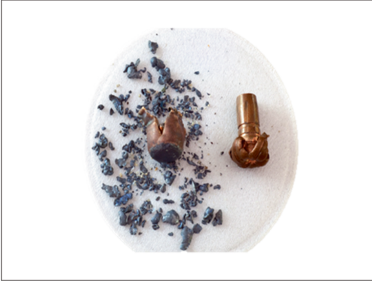
Fig. 2 The spent remains of the copper jacket and fragmented lead core of a lead-based bullet ( left ) compared with a copper (lead-free) expanding bullet that remained intact. Fragmentation of spent lead ammunition, copper jacket with lead core and pure copper. Photo courtesy of Institute for Wildlife Studies, P.O. Box 1137 Tres Pinos, California 95075
