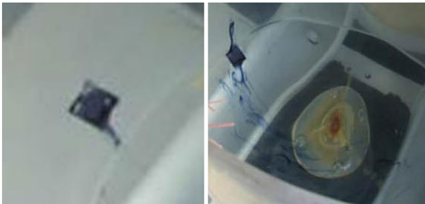
Fig. 2 Complex structure of coloured upstream and downstream ink dye wakes washed out from the plastic square marker free drifting on the surface of compound vortex cavern
