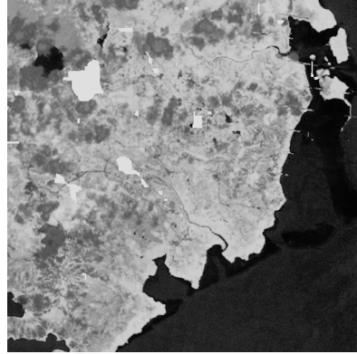
Fig. 10. NDVI, from low values (black) to high values (white), 2004/01/13, Bluecham S.A.S., NC.
