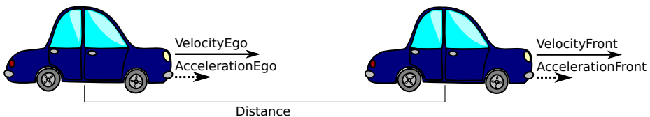
Fig. 1. Distance, velocity and acceleration between two cars.
