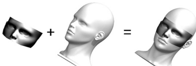
Fig. 6 Concept of surface matching. The fusion result is combined by the patient's surface ( left ) and the data obtained preoperatively by CT ( middle )
