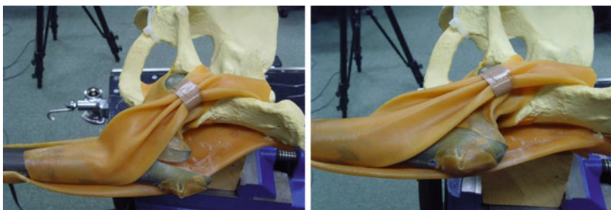
Fig. 12 Robot assisted fracture reduction with the safety features; left shows before reduction and right shows after reduction
