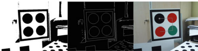
Fig. 4 The marker detection: left thresholded image, center detected contours, right detected marker
