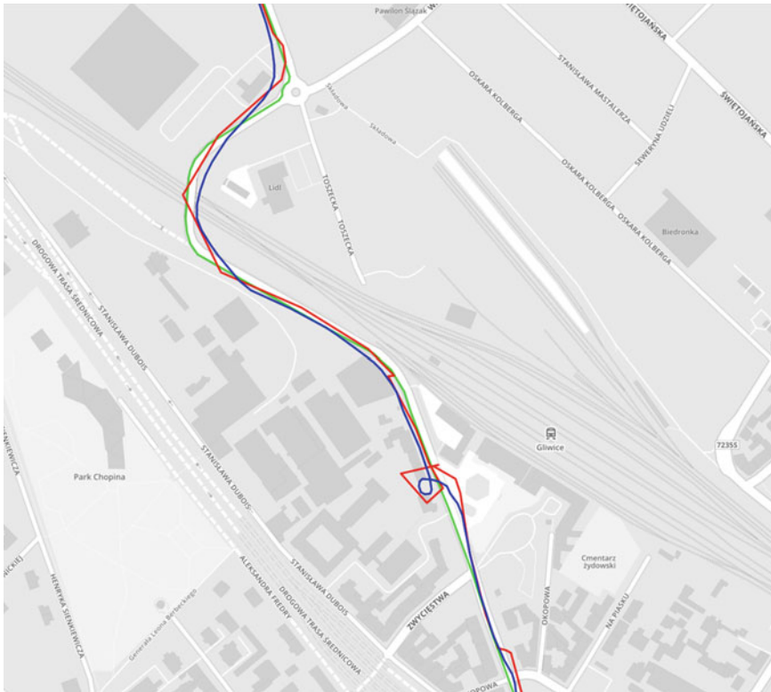
Fig. 2 Tracks example—green line is the reference track, blue line is the raw track and the red is a filtered track, map ©OpenStreetMap contributors
