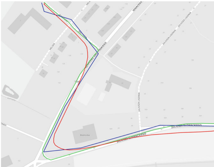
Fig. 1 Tracks example—green line is the reference track, blue line is the raw track and the red is a filtered track, map ©OpenStreetMap contributors
