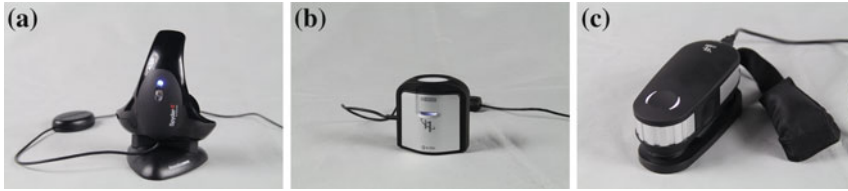
Fig. 1 Measurement devices of the calibration systems used in the research, a Datacolor Spyder4ELITE, b X-Rite i1 Display Pro, c X-Rite i1Photo Pro 2
