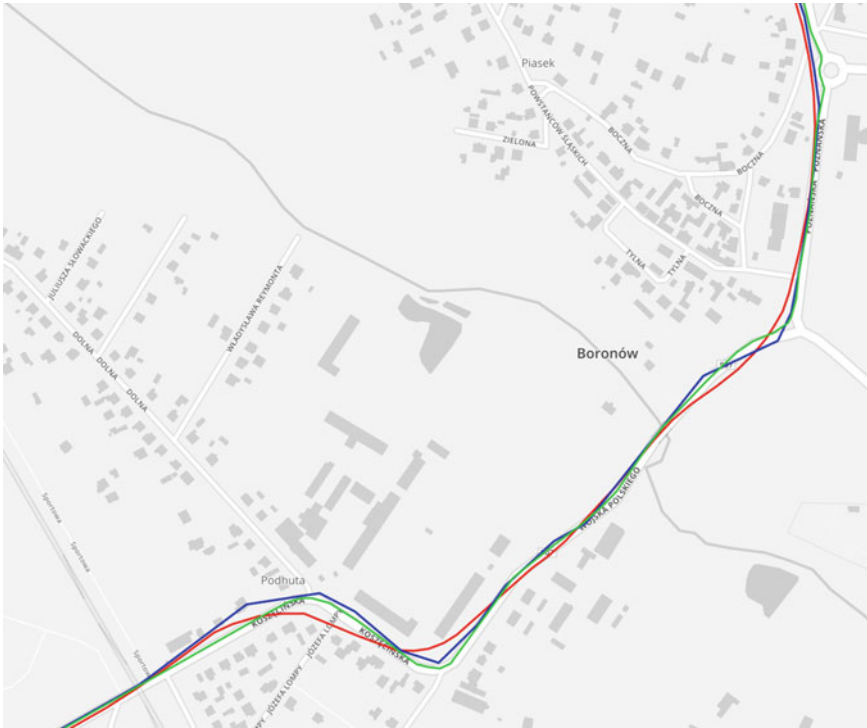
Fig. 4 Comparison of filtered and unfiltered path with multiple changes of direction, map © OpenStreetMap contributors
