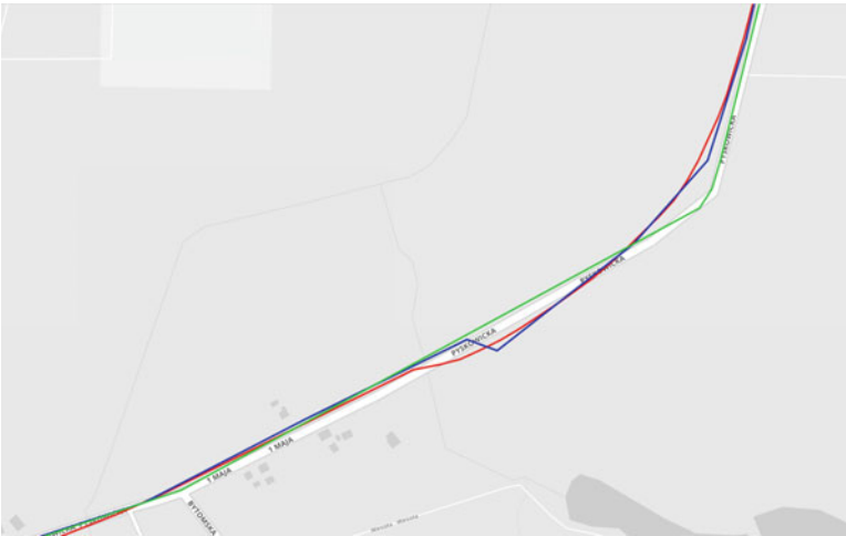
Fig. 6 Filtered and unfiltered path when error in GPS signal reception caused deviation from the real path, map ©OpenStreetMap contributors
