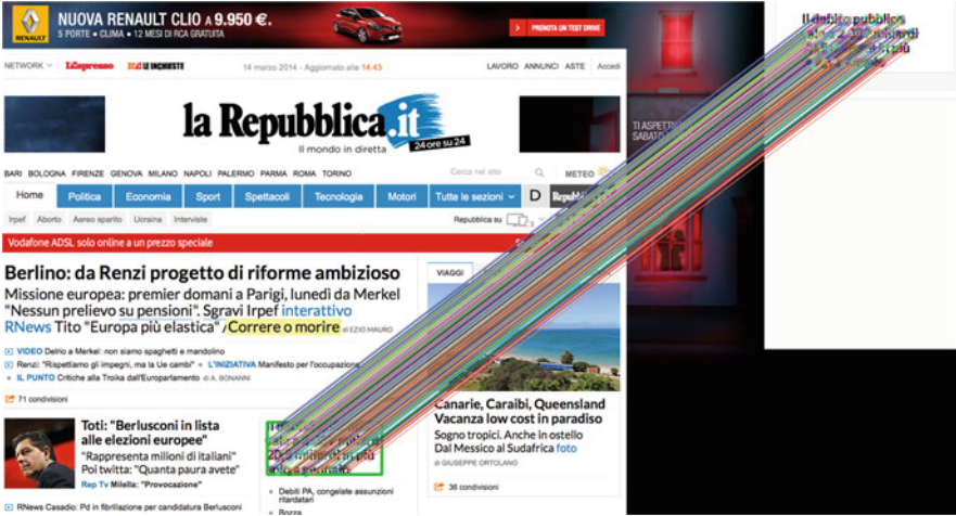
Fig. 4 Keypoint matching localization. The coloured lines track the correspondences between the keypoints, represented with thin circles . The green rectangle represents the bounding box of the news item
