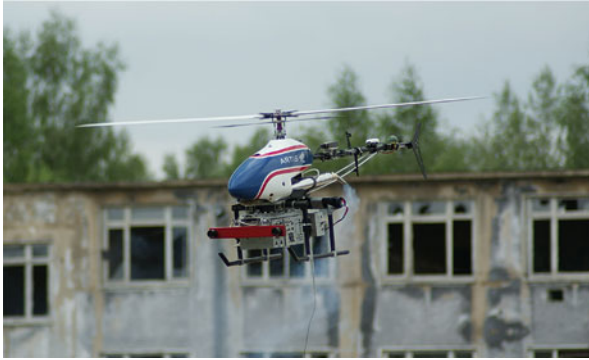
Fig. 1 Automated helicopter midiARTIS of the German Aerospace Center, maximum-take-off-weight 14 kg, rotor-diameter 2 m
