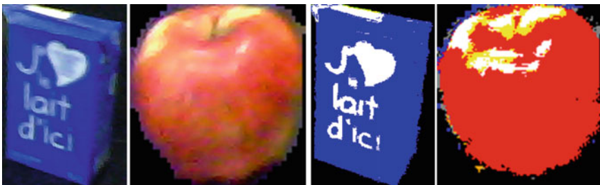
Fig. 10 Two objects observed and interpreted by the robot: the original image provided by robot's camera ( left-side pictures ) and the interpretation of those objects by the robot ( right-side pictures ). For the "apple", the robot's given description was "the object is red". For the box, the description was "the object is blue and white"
