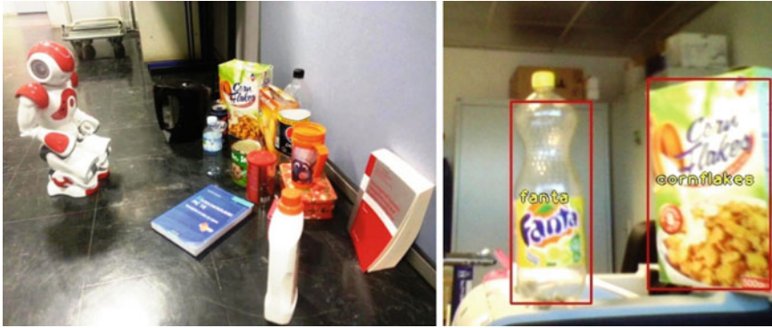
Fig. 7 Robot and the subset of collected objects used for learning ( left-side picture ) and the recognition by robot of two objects among those learned by the robot in different posture and in different location ( right-side picture )
