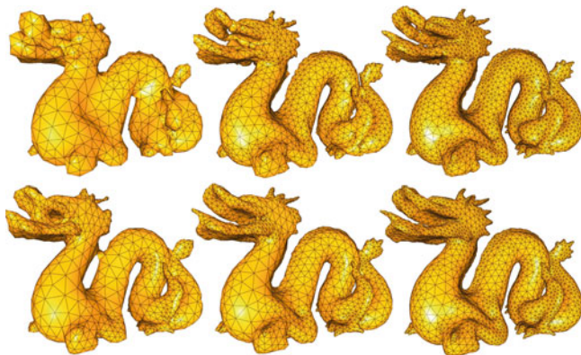
Fig. 9 A progression series of the dragon model from left to right with 2500, 5000 and 10000 triangles with the standard algorithm ( top ) and with the new algorithm ( bottom ). With the new algorithm the surface diverges faster toward the final topology
