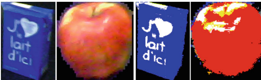
Fig. 10 Two objects observed and interpreted by the robot: the original image provided by robot's camera ( left-side pictures ) and the interpretation of those objects by the robot ( right-side pictures ). For the "apple", the robot's given description was "the object is red". For the box, the description was "the object is blue and white"
