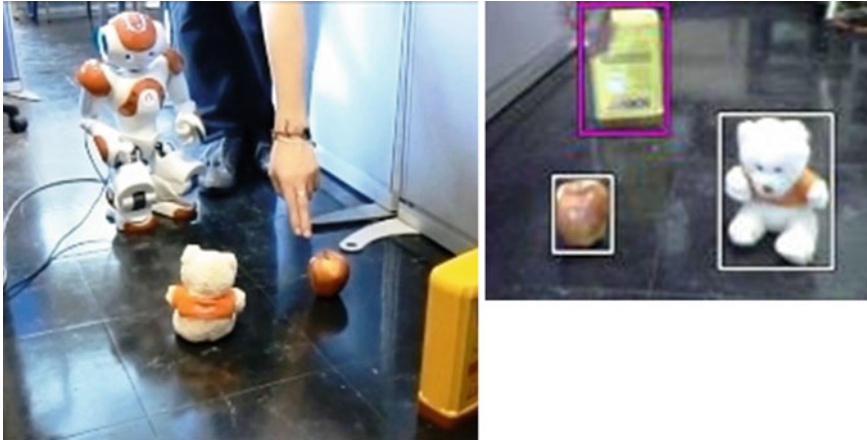
Fig. 9 Experimental setup showing tutor pointing a red apple which has not been seen before, (by the robot) asking the robot to describe that object in term of colors ( left-side picture ) and the ground truth detected objects as the robot perceives them ( right-side picture )
