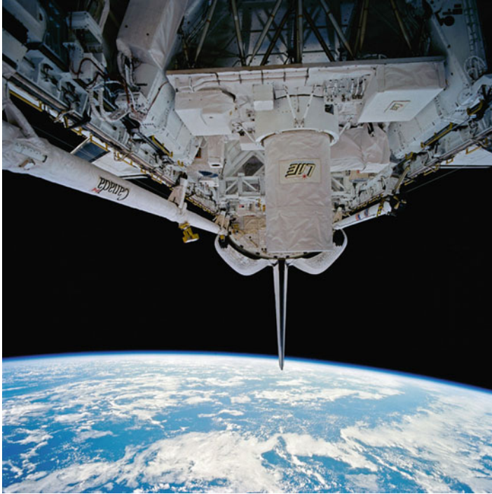
Fig. 18 The LITE LiDAR onboard the Space Shuttle Discovery (Image courtesy of NASA)
