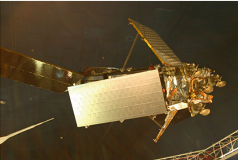
Fig. 5 A constellation of 66 Iridium satellites provides global mobile services (Graphic courtesy of Iridium)
