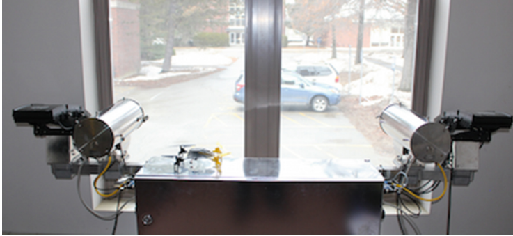
Fig. 13. Stereo-optic camera system with small quadcopter on top left corner.
