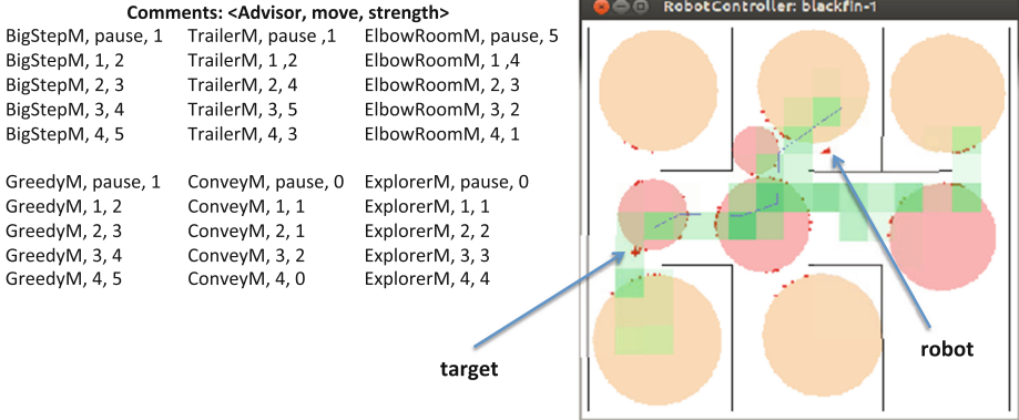
Fig. 3. A spatial model and the comments generated by the tier-3 Advisors when the robot is at the indicated decision point on its way to a target. For clarity, the walls (unknown to the robot) and only the trail selected by the Advisors are shown.
