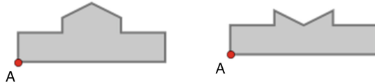
Fig. 10. Two simple shapes with a single different vertex. Vertices are labeled counter-clockwise from the start vertex A. Here, the vertex which differs the most is vertex F on the "top" of the shape.
