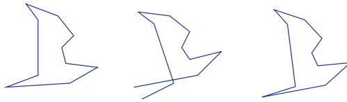
Fig. 8. 10-vertex representation of a bird. The final polyline (right) exhibits both some skew and scale deviations from the initial polyline (left). However, both the input and final polylines have the same eOPRA_8 direction hull descriptions.
