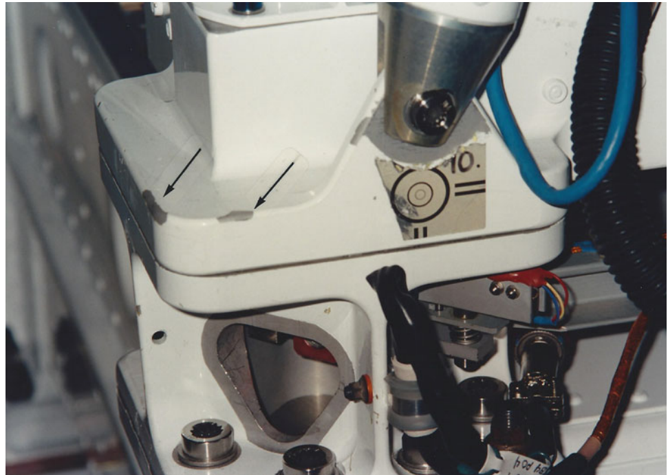
Fig. 8.44 Detail, showing some small areas of Chemglaze white paint removed from rounded corners, indicating the need to check the suitability of the primer. All other areas coated with Chemglaze (also external and on Pallet) were in excellent condition
