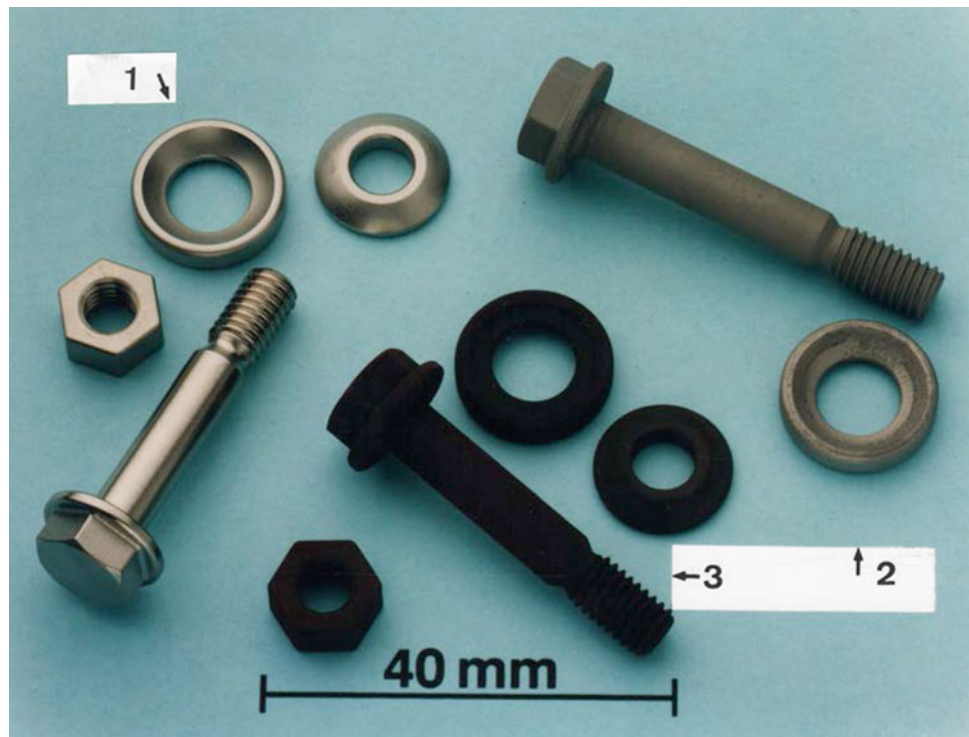
Fig. 8.32 Silicide-coated fasteners developed for assembly of the Thermal Protection System of re-entry vehicles. These oxidation-protected fasteners are machined from niobium alloy 752. After machining (1) the parts are coated with SiCrFe and annealed (2). The arrow at (3) shows the pre-oxidized deliverable finish. These fasteners have been tested at elevated temperatures and do not degrade in mechanical properties following exposure in air to 1150 °C for more than 500 h. They also survive temperature cycling to 1300 °C for 40 h (Courtesy of Plansee Aktiengesellschaft)
