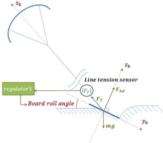
**Fig. 8** Board course regulator block diagram
