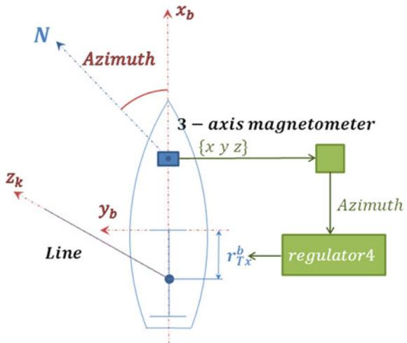
The third regulator presented on Fig. 7 is used for board drowing stabilization. Control parameter is kite line tow force. It should compensate board hydrodynamic force correspondent component. Control action is line fulcrum transverse shift. Time delay for the regulator should be higher than kite position regulator to implement the independency of regulations. The regulator should set correct board attack angle when kite position is set.
