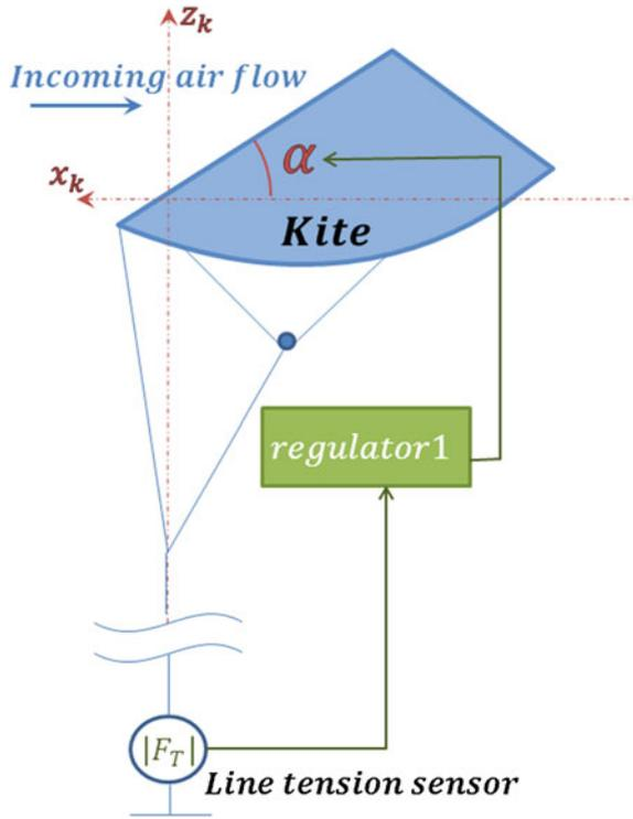
Fig. 6 Kite elevation regulator block diagram
