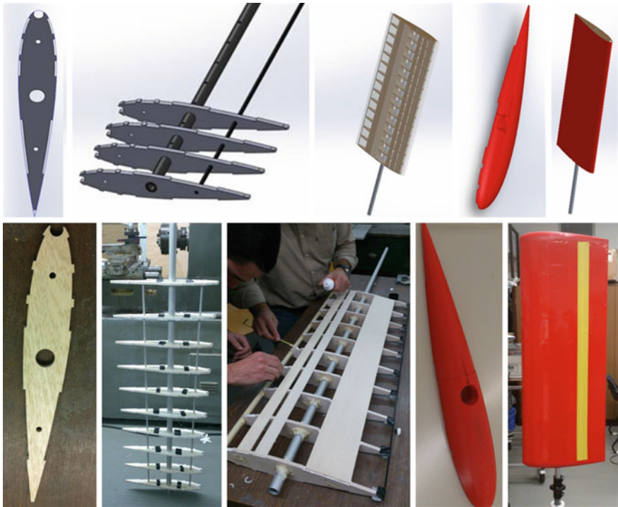
Fig. 2 Different stages of the construction of the wing sail prototype, from the CAD drawings to the final result
