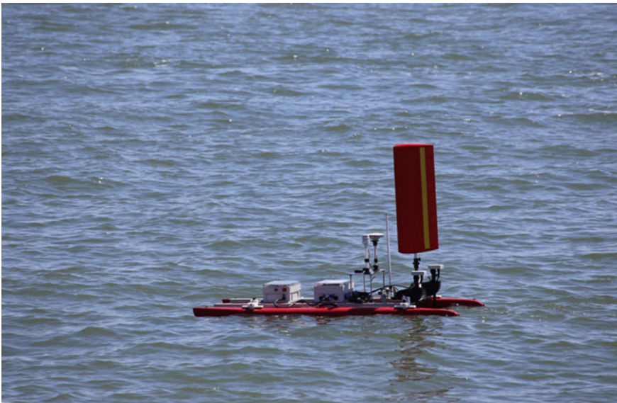
Fig. 6 Zarco being tested with a single wing sail at the stern
