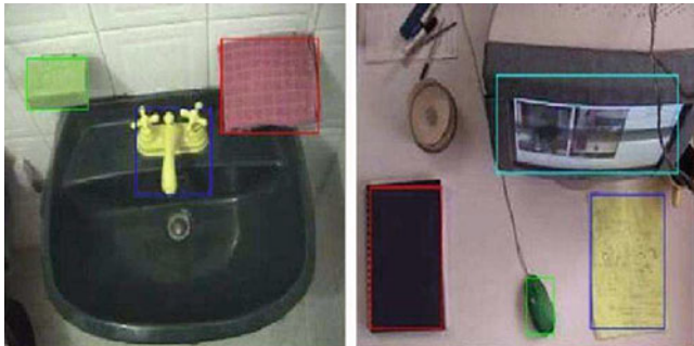
Fig. 8.2 Example of object detection in two domains. Left image : washstand. Right image : office environment. Each object detected is highlighted and closed in a rectangle
