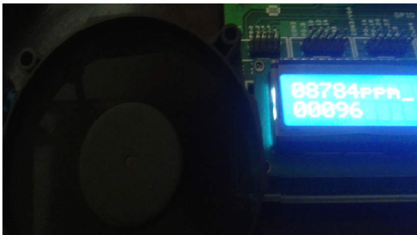
Fig. 9 Real time LCD display of 8784 PPM along with running fan
