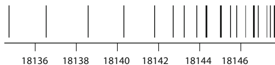
Fig. 2.20 Rotational spectrum in the 0–0 band of ^{35}\text{Cl}_2
