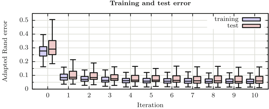
Fig. 4. Adapted Rand error for random forest trained with the given number of iterations. Iteration 0 is from the initial random forest trained with a few strokes for membrane and intracellular space. The segmentation error is evaluated for each slice and the distribution over the stack is shown.
