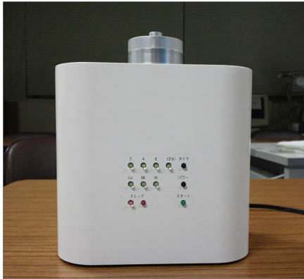
Fig. 1 The nano-mist sprayer
