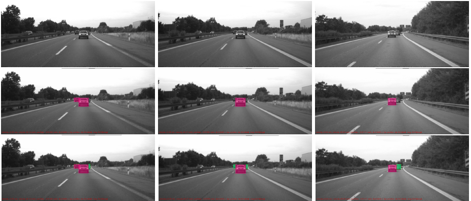
Fig. 2. Top: Input frames (intensity channel). Middle: A tracked vehicle acts as occluder (pink rectangles). Bottom: Tracked occludees (green rectangles) and occluders (pink rectangles).
