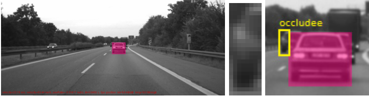
Fig. 1. Left: A sample frame with a tracked occluder (the filled pink rectangle). Middle: A partially-visible car. Right: Zoom-in view on an occludee (the yellow rectangle).
