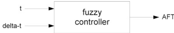
Fig. 7.15 Temperature and Delta-temperature are the inputs to the air-conditioner controller. The output is temperature and air flow, AFT
