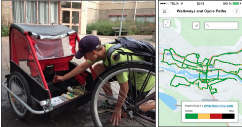
Fig. 3. Left: Roadroid installation; Right: Walkways and Cycle Paths Mobile e-Service
