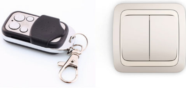
Fig. 5.3 Remote control and wall switch of a smart home system, representing two different designs of one and the same technical component
