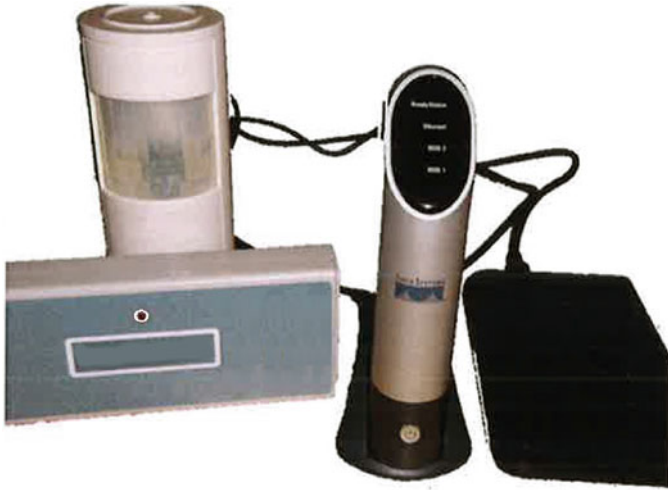
Fig. 7.2 The customized central unit running independently on the basis of the Gateway component, a Network Bridge in combination with a harddisk exchanging the PC and a Motion Sensor as example component [3]
