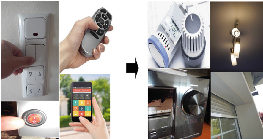
Fig. 5.2 Different forms of interfaces in a smart home and devices that can be controlled by them
