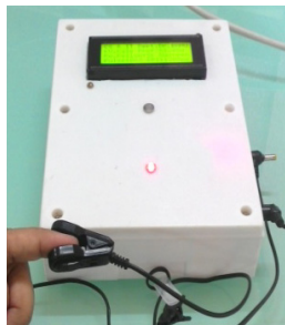
Fig. 3 IR Based Pulse detection Sensor with the measuring Unit
