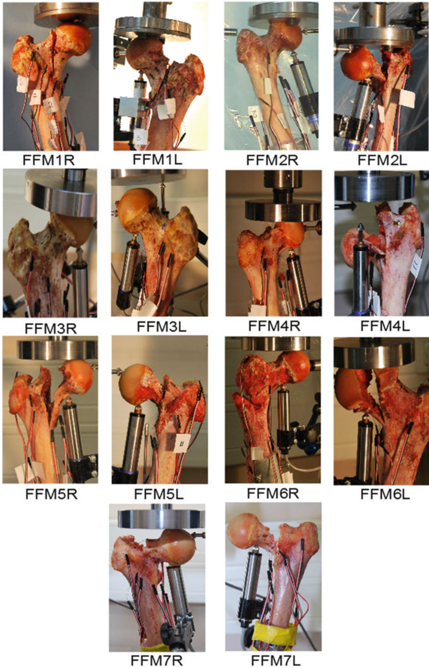
Fig. 5 Fracture patterns in femurs with metastatic tumors. Figure from [19]
